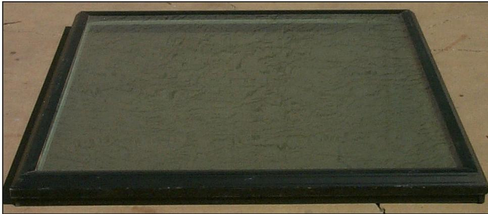
Figure 19. Double-glazed low-e flat skylight – Type A
